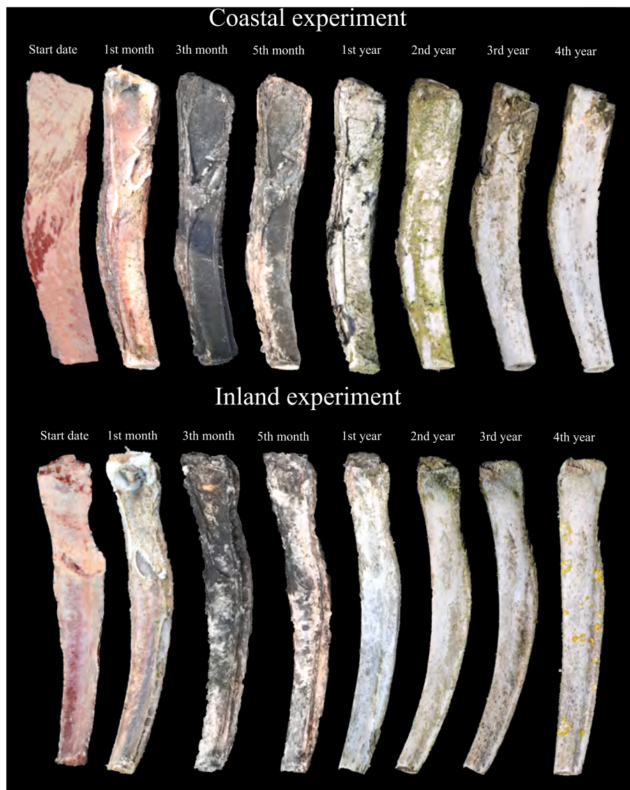
Fig. 4. Monitoring of a specimen control from the coastal and inland experiments during the first four years of the experimentation.
